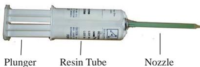
Before applying to the quick disconnect, use the plunger to evenly push out a small amount of resin to get a proper mix of the 2-part epoxy. Then apply resin into the housing, enough to cover the wires and contacts. The resin should be about 3mm onto the cord jacket. Note: Adding too much resin may cause excess to be forced into the female end of the pin
