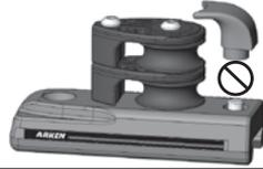
Use allen wrench to remove two screws holding sheave assembly. **Do not remove deadend horn.** Capture splice on horn and assemble sheave using threadlocking solution such as blue Loctite® on screws. When using smaller control line pass eye inside horn and run tail through to make a hitch without removing sheave assembly.
