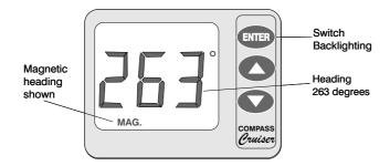
Figure 2 - Normal operation display
