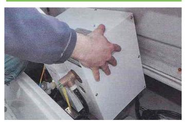
The compactness of the casing, measuring just 330 mm wide, 350 mm high and 340 mm deep, will fit nicely in a narrow compartment, here located under the rear seat.
