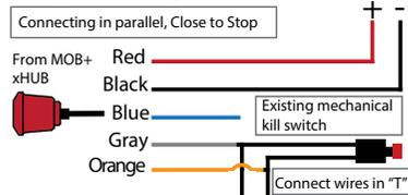
MOB+ can be installed together with your existing kill switch by connecting it in series or parallel. If you should connect in series or parallel depends on your existing kill switch function. The above picture shows an example with Close to Stop connection.
