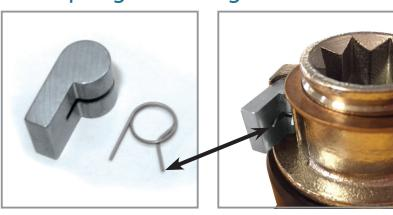
Note the orientation of the bent spring "arm"
